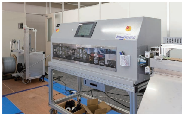
Auto wire skinning machine for automatic cable cutting and terminal processing
