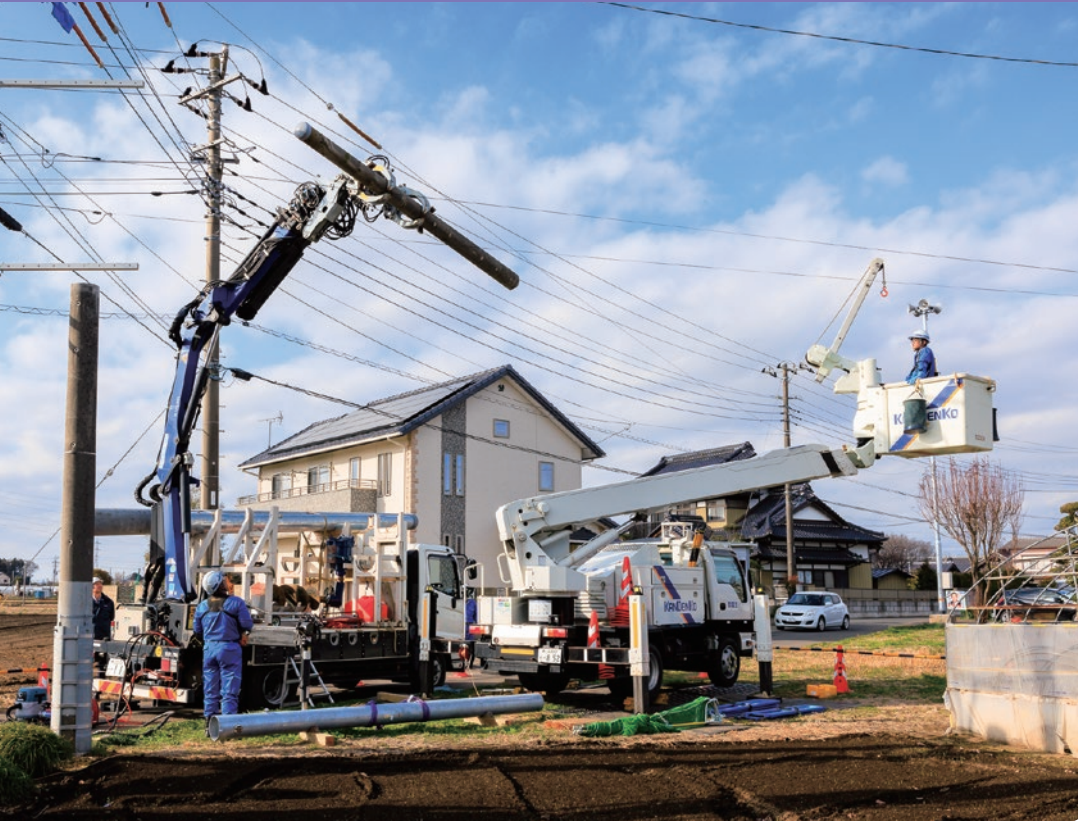
Field testing of next-generation pole-setting vehicles capable of transporting, excavating, and installing power poles with a single vehicle (Ibaraki Prefecture)
