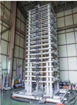
▲Research & Development Institute ◀1,800kV impulse voltage generator
