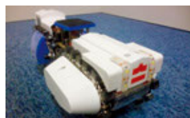
Self-propelled ceiling wiring robot
