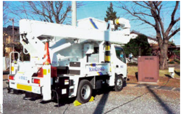
Battery-operated aerial platform vehicle
